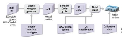
FIGURE 2 Automated process to build a virtual ECU (© QTronic)
