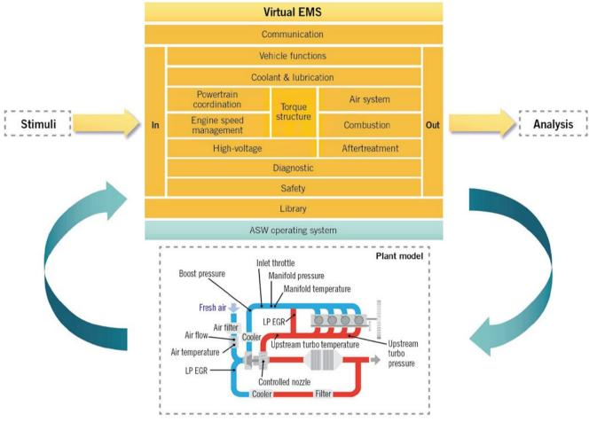
FIGURE 3 Virtual ECU of Renault EMS connected to engine model (© QTronic)
