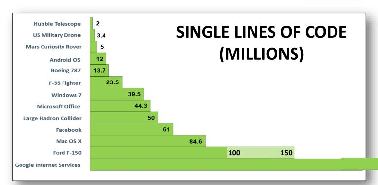
Modern automotive vehicles contain between 100-150 million lines of code across 30-80 networked ECU's with up to 30,000 physical parts, making them one of the most complex engineered systems in the modern world.
